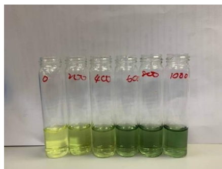
Figure 2.14: Standard gallic acid solution after adding 7.9 mL of distilled water and 500 μL of Folin-Ciocalteu reagent.
