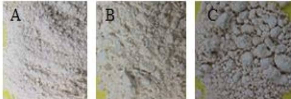
Figure 1.0 Physical properties of powdered particles at (A) 75 \pm 2^\circ\text{C} , (B) 80 \pm 2^\circ\text{C} and (C) 85 \pm 2^\circ\text{C} air outlet temperature of spray dry.
