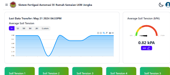
Figure 4: Development of a dashboard platform for monitoring and control of the fertigation system at nursery CRDC Jengka
