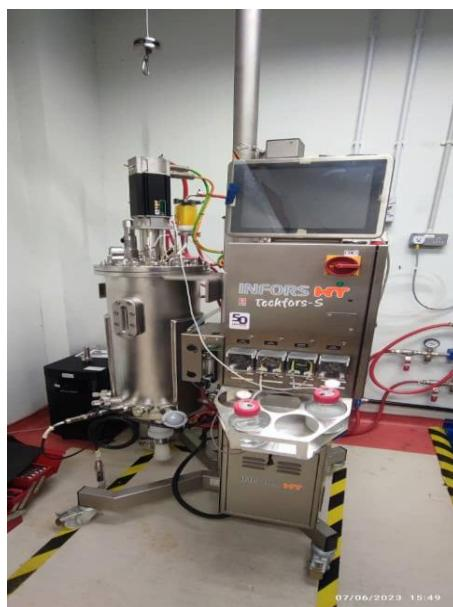
Figure 1. The growth of selected endophytic bacteria using 30 L Bioreactor (Techfors; Infors, Switzerland).
