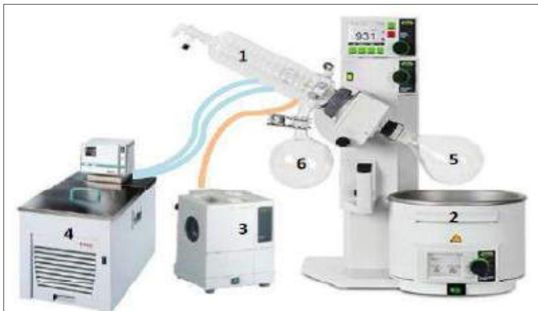
Figure 1.1. The Rotary Evaporator, Buchi R-250V as a roaster unit.
