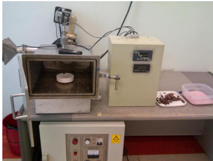
Figure 1: The microwave laboratory dryer experiment set up
