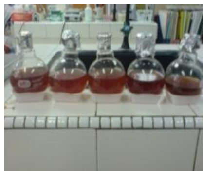
Figure 2.4 Aqueous extract for freeze drying for laboratory methods of preparation of cocoa polyphenol extracts
