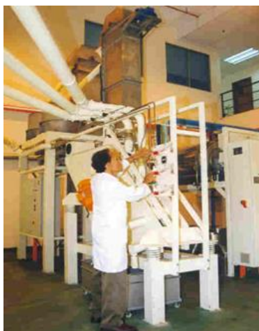
Figure 2.13 Cocoa beans deshelling for the pilot scale method preparation of cocoa polyphenol extracts
