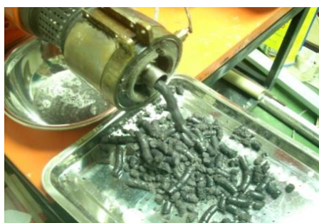
Figure 2.14 Defatting nibs for the pilot scale method preparation of cocoa polyphenol extracts
