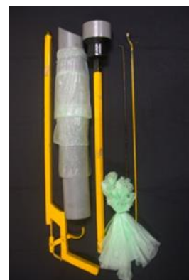
Figure 11 : DINAMIK Pod Sleever for pod sleeving
