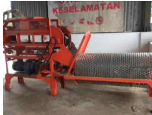
Figure 14 : COBRE ® , a machine for cocoa pod breaking and bean separation
